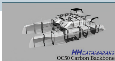
The hulls and superstructures of the Ocean Class are made of a glass/thermoformed foam/vinylester sandwich. A carbon frame takes up the forces. The shipyard's expertise in the mastery of composite materials is excellent.
