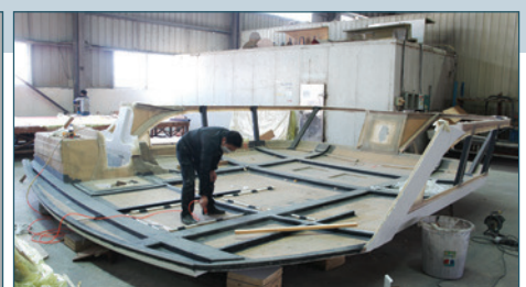
The hulls and superstructures of the Ocean Class are made of a glass/thermoformed foam/vinylester sandwich. A carbon frame takes up the forces. The shipyard's expertise in the mastery of composite materials is excellent.
